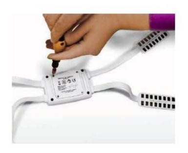
A cross-head screwdriver, such as a No.1 Phillips Head or Pozidrive to screw the backplate onto the Control Unit.
